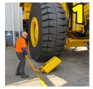
To move into position, pull the handle down, levering the Workshop Wheel Chock onto its back wheels.
