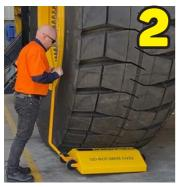
Lift the Workshop Wheel Chock onto its front wheel and bring close to the tyre. Bring the back of the chock around into position.
