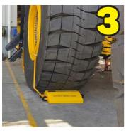
When chocks on both sides of the wheel are in position correctly, the truck is secured.
